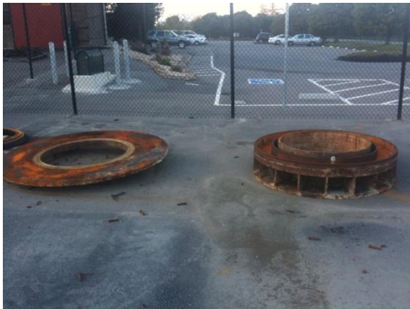
Original base & turntable, Biotower No. 2
